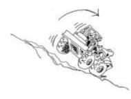
Operate up and down slopes where a rollover hazard exists.
