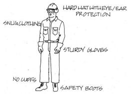
When working around a chipper, specific Personal Protective Equipment should be worn.
