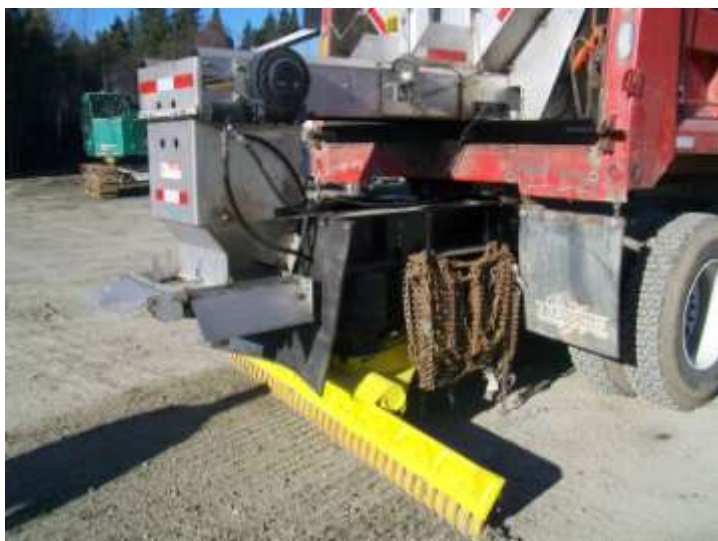
Fig. 2 Completed scarifier mounted on plow truck.
