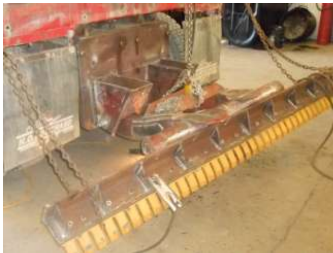
Fig. 1: Scarifier under construction.
