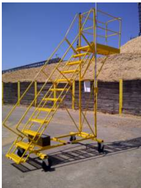
Fig. 2: Mobile tarping platform/ladder for chip/residue receiving/unloading facilities.
