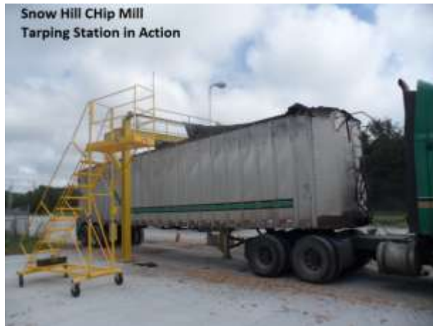
Fig. 3: Tarping station in use.
