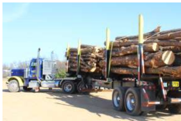
Fig. 3: Four Luftmans on this trailer—one for each bolster.
