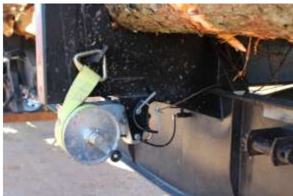
Fig. 1: Close-up of tensioner/drum. Binder strap is wound into the drum and hangs up when not in use.
