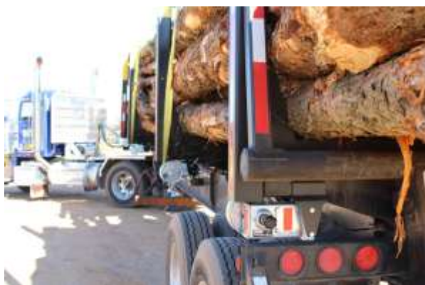
Fig. 2: Photo shows placement of four tensioner drums and air valves.
