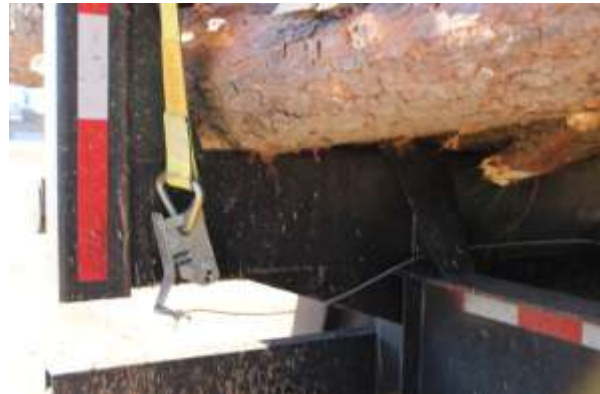
Fig. 5: Close-up of strap connected to the deployer, which is mounted on the bunk or frame (passenger side).
