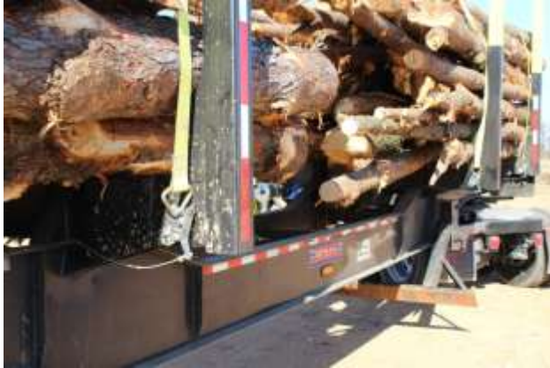
Fig. 4: Passenger-side view. The quick-release locking mechanism is remotely operated and controlled from the driver's side, so the driver does not have to walk around the load while unbinding—a safety advantage!
