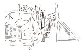
If an unbinding station is not provided, do not loosen binders without support of an unloading machine (clamped over the load) unless the logs are clearly below the bolsters and supported by at least two standards.
