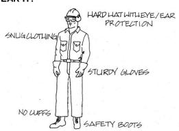
When working around a chipper, specific Personal Protective Equipment should be worn.
