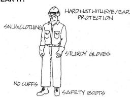
When working around a grinder, specific Personal Protective Equipment should be worn.
