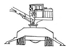
Before climbing to operator's station, check steps, walking, and working surfaces to ensure they are clear of oil, grease, fuel, mud, snow, ice, and debris.
